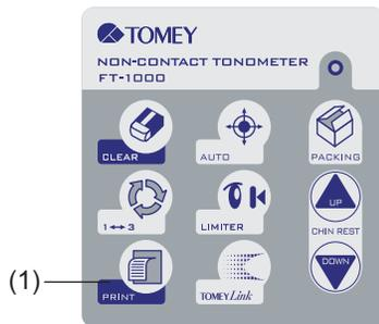
After the measurement, touch the "PRINT" button to print the data.
