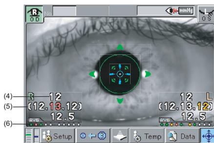
The latest measurements (4) appear in the lower left of the screen. Three new measurements (5) appear under the latest data.
