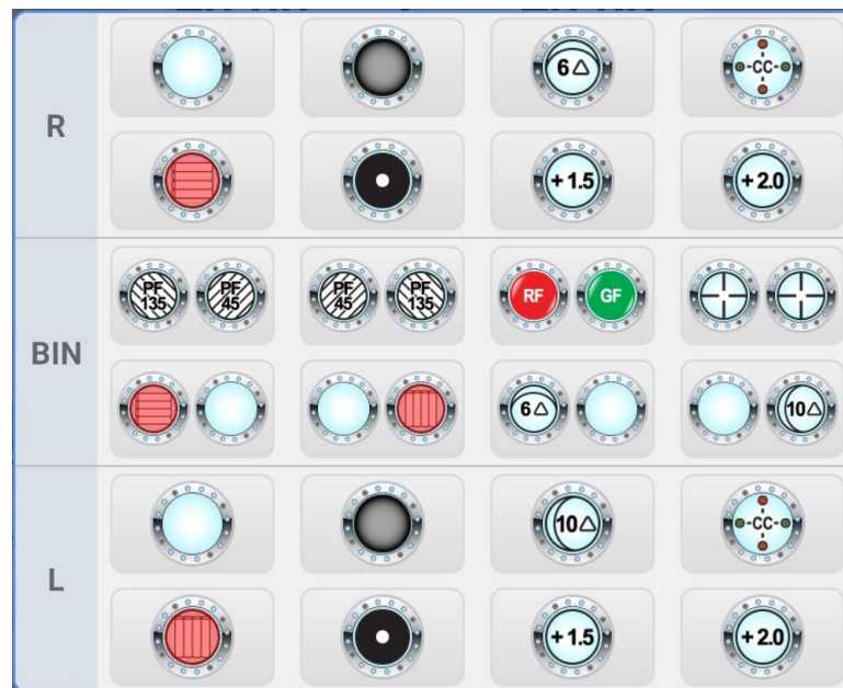
[Figure 5-9] Auxiliary lens for right eye, Left eye and Binocular eye
