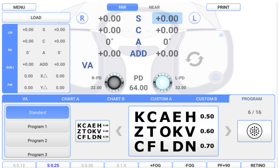
[Figure 9-7] Adjustment of the S-C-A Value
