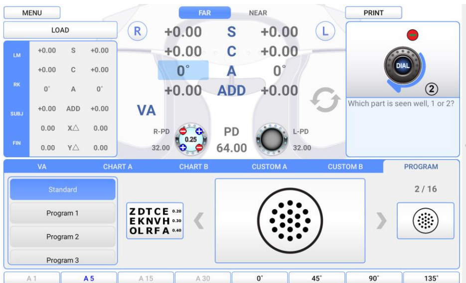
[Figure 9-3] 2 nd step Cross Cylinder Test (Axis)
