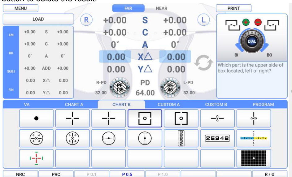
[Figure 10-19] Horizontal Coincidence(Aniseikonia) Test
