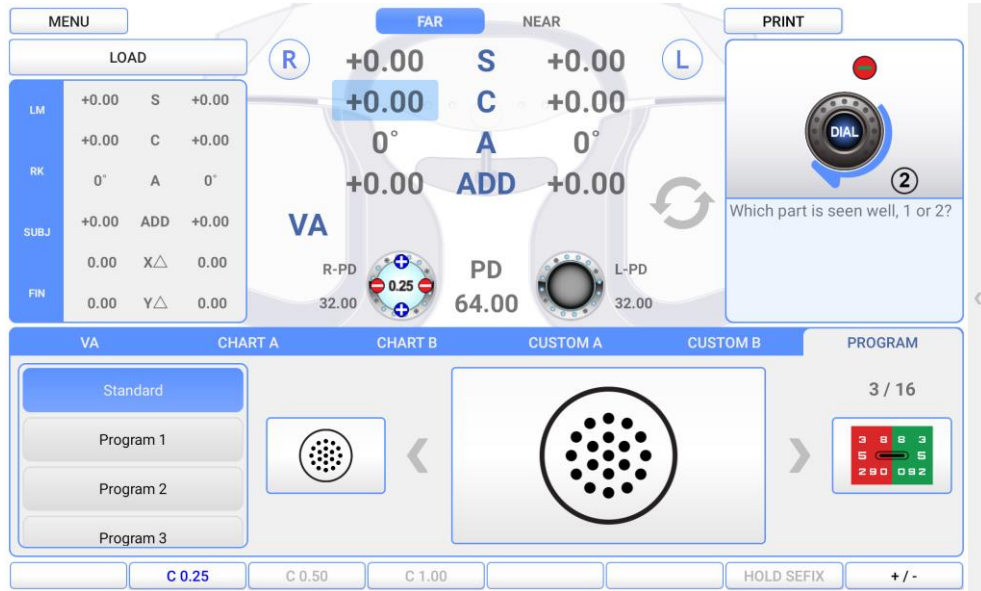
[Figure 9-4] 3rd step Cross Cylinder Test (CYL)
