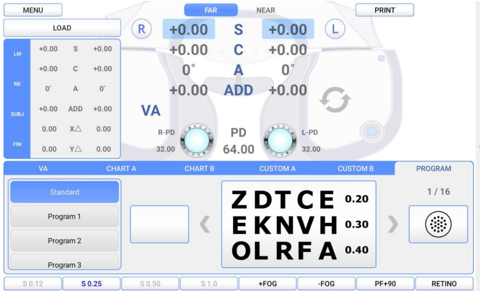
[Figure 9-2] Adjustment of 1 st step S - C -A Value
