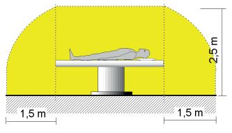
The patient area is the volume defined as shown in the figure, within which the patient may come into contact (intentionally or unintentionally, directly or through contact with the operators) with medical electrical and other devices making up the system
