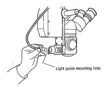
Insert the other side of the light guide into the mounting hole. And tighten the screw.
