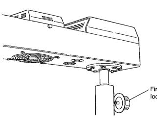
Tighten the first arm rotation lock knob of column.
