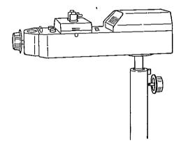
Level the first arm and insert the first arm gently in the column.
