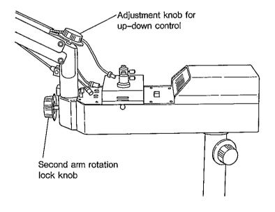
Tighten the second arm rotation lock knob lightly.
