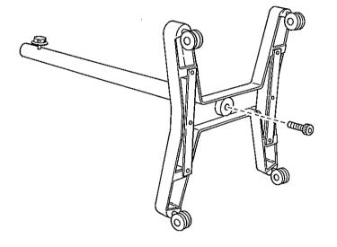
Screw manually "Bolt with a Hexagonal Hole" and secure with hexagonal spanners.
